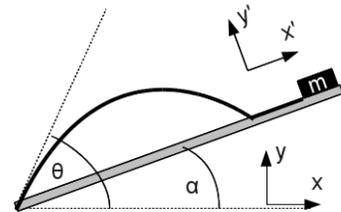
Figure 3: Mass on incline with friction.
