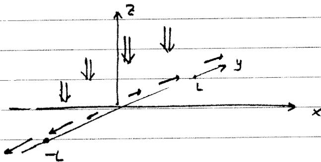
Note cross-isobaric flow (in  $y$ -direction) directed away from high pressure core in  $y=0$ . Magnitude of this flow increases from  $y=0$  to  $|y|=L$ , for  $|y| > L$  constant
